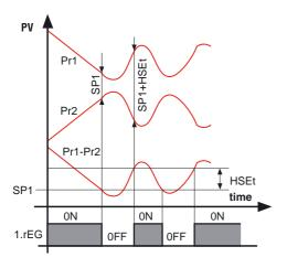
Example of differential ON/OFF control (On.FA) with "Func"= CooL
