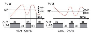
The control works in the following way: in the case of reverse action, or heating ("FunC"=HEAt), it deactivates the output, when the process value reaches [SP + HSEt] in case of symmetrical hysteresis, or [SP] in case of asymmetrical hysteresis and is then activated again when the process value goes below value [SP - HSEt].
