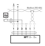
Requirements for switching contact: The switching contact must be able to accurately switch a current of 16 mA @ 24 V.
