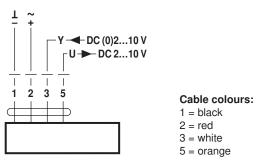
Override control (frost protection circuit)
